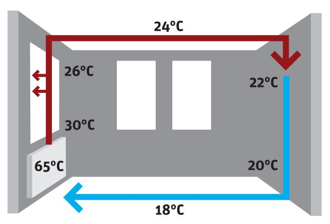
Inlet temperature: 65 °C Room temperature: 22°C
